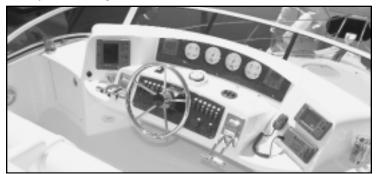
The helm has easy-to-read black-on-white gauges and room for basic electronics.
